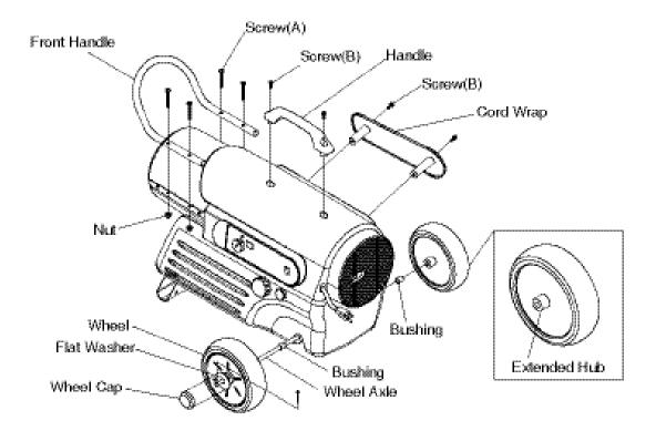
Figure 8. Wheel and Handle Assembly, RMC-KFA120TDLX/RMC-KFA170TDLX Models Only.
